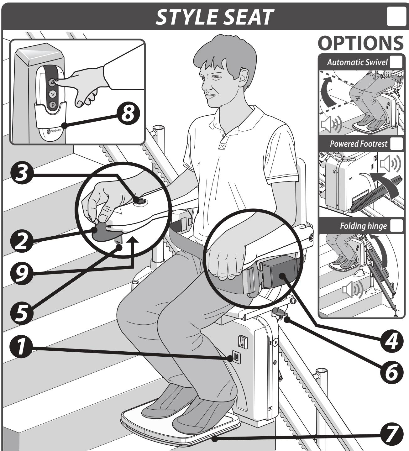
The illustration above shows the features used to operate the STYLE seat. The STYLE seat can be upgraded with the Automatic Swivel seat, Powered Footrest and the Folding hinge, options to create even more seat comfort and user-friendliness.
