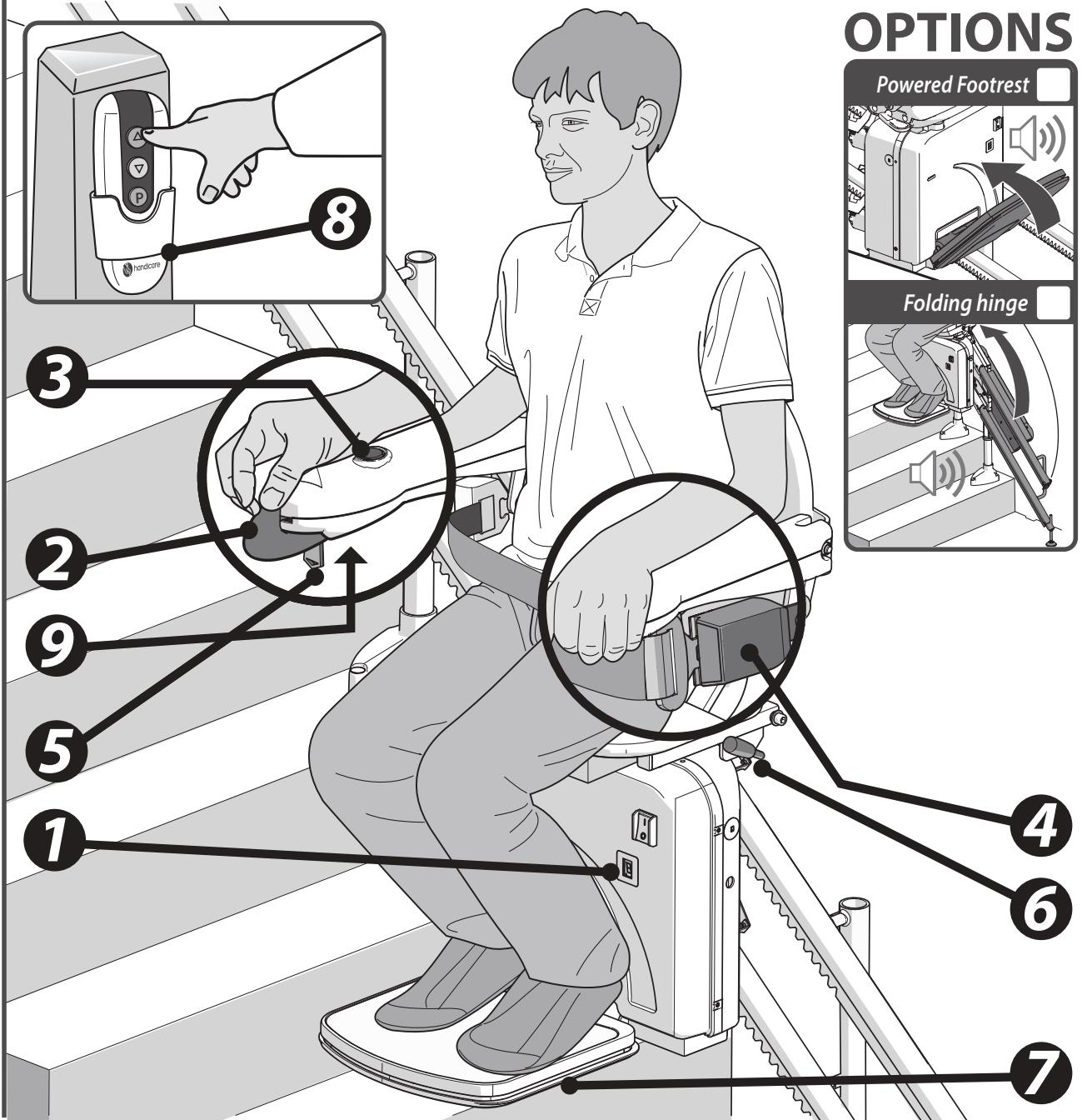
The illustration above shows the features used to operate the SIMPLICITY seat. The SIMPLICITY seat can be upgraded with the Automatic Swivel seat, Powered Footrest and the Folding hinge, options to create even more seat comfort and user-friendliness.
